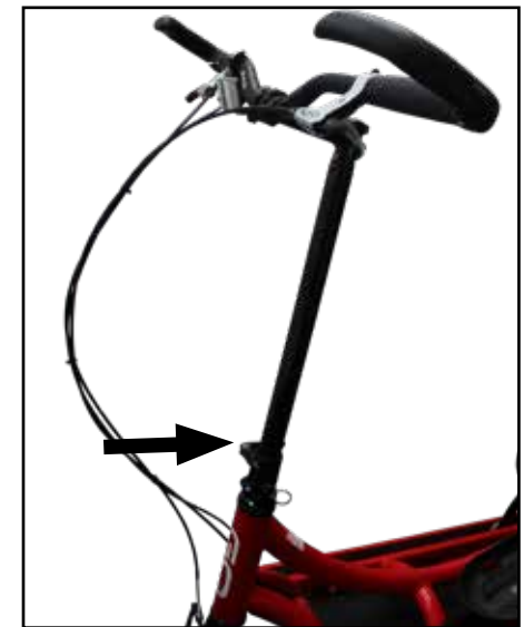
Left: Location of quick release lever on front wheel. Below: Locations of quick release levers on steering columns.
